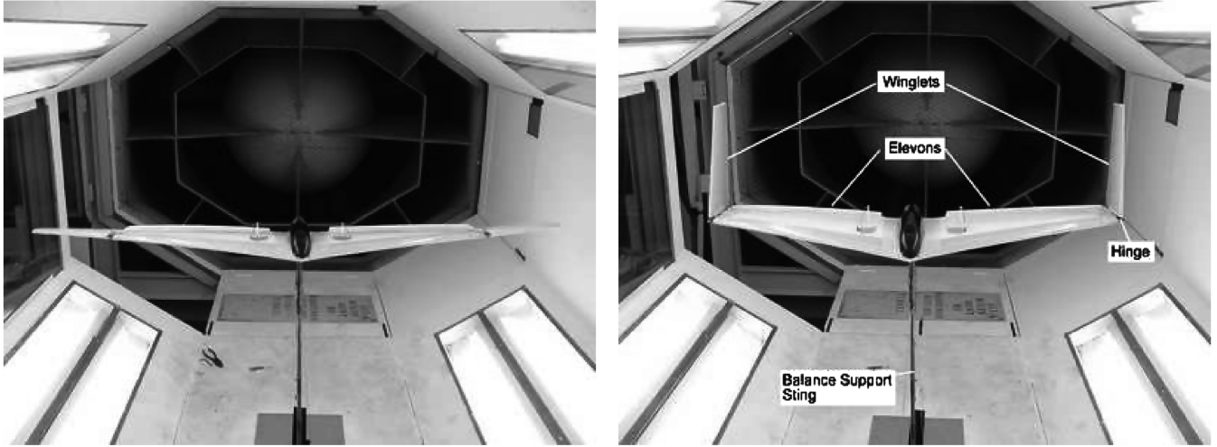
Fig. 3 Experimental model as mounted in the wind tunnel; left: both winglets planar; right: both winglets upright.
